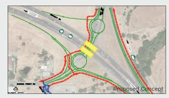
movement of vehicles. The two roundabouts will be located on Highway 221 north of Highway 29 and on Soscol Ferry Road south of Highway 29. The roundabouts will allow drivers to turn on and off the highways. The project will also construct 1,200 feet of class 1 facility to accommodate bicycles and pedestrians through the intesection.
